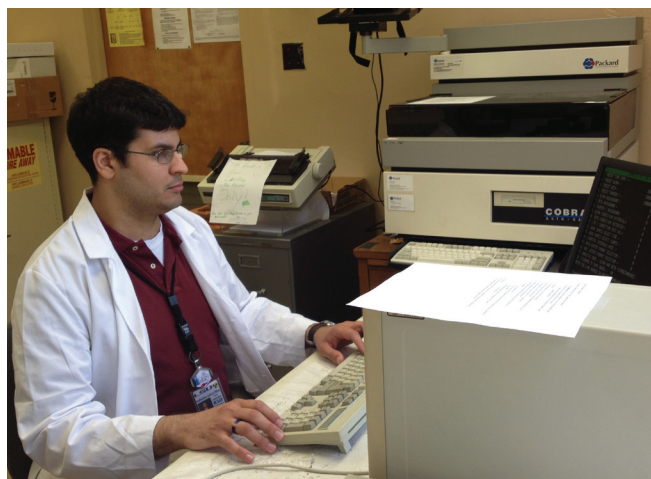
RSO Radiation Specialist Amin Hamideh examines the results from leak tests of sealed radioactive sources using a proportional counting system.
